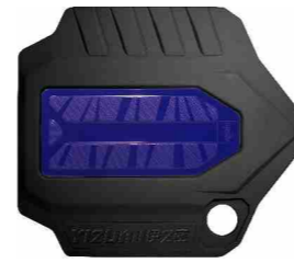
Product: Engine Cover Molds: InPUR 1+2 innovative molds Machine: UN500DP Two-platen Injection Molding Machine Material: AKROMID® B3 GF 15 1 black + SHGPuR Part size (LxWxH): 400x350x25 mm Part weight: 470g Cycle time: 60s
